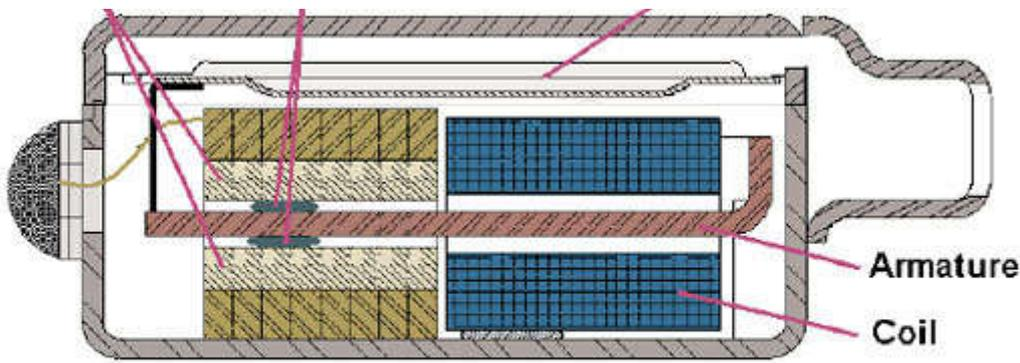
Figure 1: Cross-section of the Knowles FED receiver (i.e., ferrofluid-damped ED receiver)
