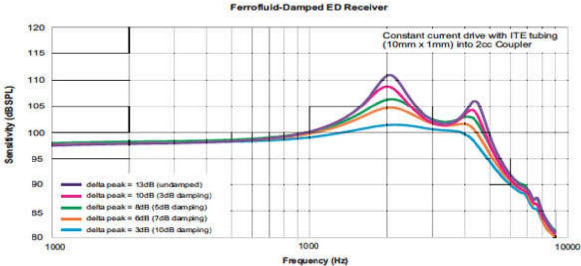
Figure 3: Frequency response curves under constant current drive conditions for fluid-damped FED receivers and a response curve for an undamped ED receiver. Labels in legend are the delta peak values.
