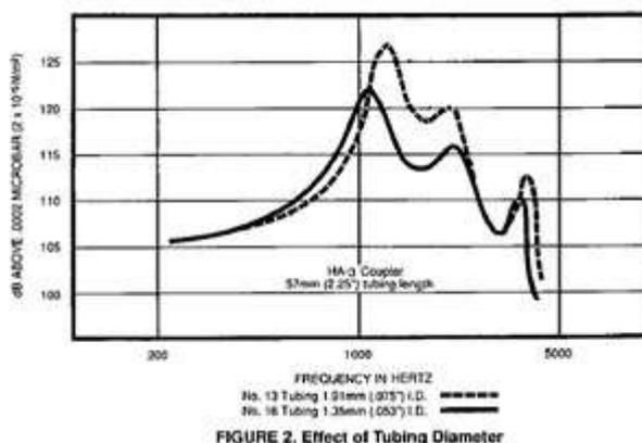
FIGURE 2. Effect of Tubing Diameter
