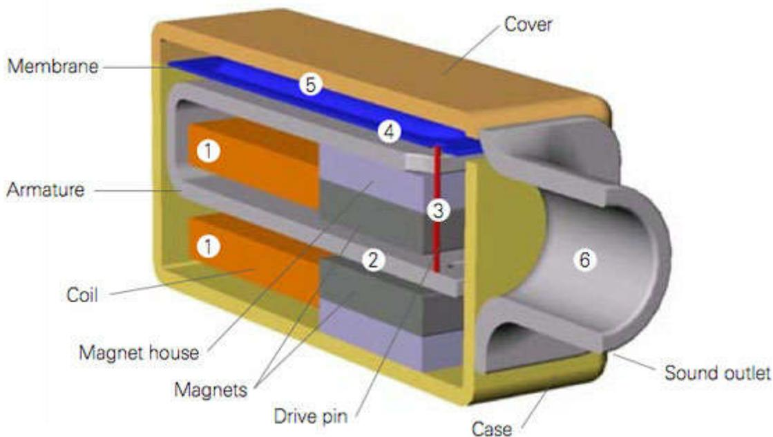
Generalized illustration of a balanced armature receiver.
