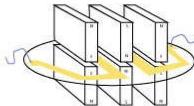
Diaphragm in place with conductive trace (yellow) immersed in areas of isodynamic field.
