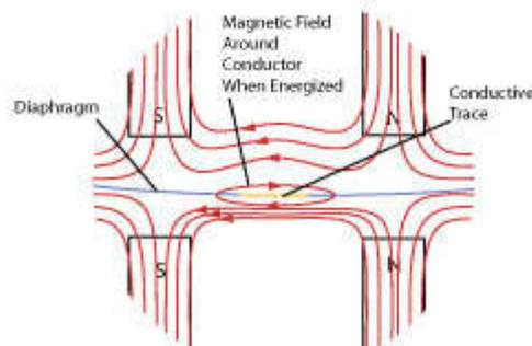
Magnetic field induced by electrical current flow around conductive trace pushes diaphragm away where magnetic flux arrows are opposed; pulls where arrows align.
