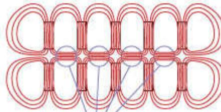
Arrays of magnets form multiple regions of isodynamic magnetic field.
