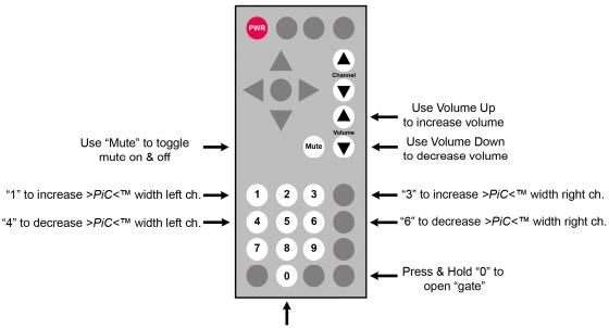
Use "2", "5", &"8" to adjust >*PiC*<™ width of both channels at the same time "2" increases width & "5" decreases width "8" resets >*PiC*<™ width to normal
