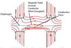
Magnetic field induced by electrical current flow around conductive trace pushes diaphragm away where magnetic flux arrows are opposed; pulls where arrows align.
