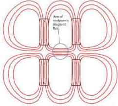
Proper magnet geometry creates an area of evenly distributed force: an isodynamic field.
