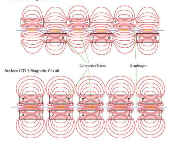
Engineers are pretty good at finding a variety of solutions to a probem, so there are also numerous other configurations of magnetic circuits in planar-magnetic headphones.
