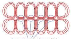
Arrays of magnets form multiple regions of isodynamic magnetic field.
