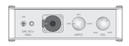
**DAC 1866 OCU** is a Hi-Fi digital-to-analogue audio converter. In accordance with Russian state standard specification 24388-88, its output amplifier belongs to zero (highest) complexity group. The device is based on precision 16-bit R2R DAC from Analog Devices – AD1866.
