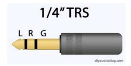
The 1/4" TRS (aka 6.25mm TRS for the metric folks) is the most ubiquitous plug for home/studio headphones. The tip is left signal (L), the ring is right signal (R), and the sleeve is ground (G).
