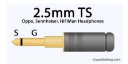
The 2.5mm TS with narrow shoulders originally was created for use with the Sennheiser HD700 headphone cups, but now has also been adopted for the Oppo PM-1, Oppo PM-2 and can potentially be used with the HiFiMan 400S, HE-560, HE-1000 and Edition X as the stock TRS does not use the ring (R). The tip is used for signal/positive, and the sleeve is ground/negative.
