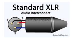
The standard-sized XLR is used for a few different applications. As an audio interconnect, Pin 1 is the ground, Pin 2 is the positive signal, and Pin 3 is the negative signal. You'll notice that most XLRs have the pins labeled 1, 2 and 3 if you look closely enough.
