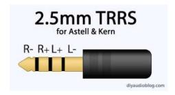
The 2.5mm TRRS is commonly used for balanced operation for **Astell and Kern** portable digital audio players. Tip is right negative (R-), ring closest to tip is right positive (R+), ring closest to sleeve is left positive (L+) and sleeve is left negative (L-).
