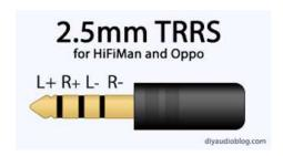
The HiFiMan HM-801 digital media player and Oppo PM-3 headphone (balanced) follow this unique configuration using the 2.5mm TRRS. Tip is left positive (+), ring closest to tip is right positive (+), ring closest to sleeve is left negative (L-) and sleeve is right negative (R-). Get yourself a nice aftermarket cable using the TRRS from Zynsonix Audio.
