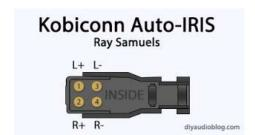
The Kobiconn Auto IRIS is an odd little connector typically used with cameras. These are found on Ray Samuels (RSA) balanced portable headphone amplifiers like the Protector and SR-71B, however are also on amplifiers Centrance GloveAudio A1, HiFi M8, and the ALO Rx Mk3 B. Pin 1 is left positive (L+), pin 2 is right positive (R+), pin 3 is left negative (L-), and pin 4 is right negative (R-).
