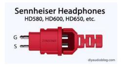
The Sennheiser HD connector features two pins. It's difficult to notice on a quick glance, but one is larger than the other. The larger pin should be used for ground/negative, and the smaller pin is signal/positive.
