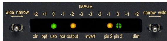
Hint: To double-check if the setting is correct, use the  $\longleftrightarrow$  switch to move the cursor away from the setting you just changed to see if its LED indicator is “On” or “Off” (instead of flashing).
